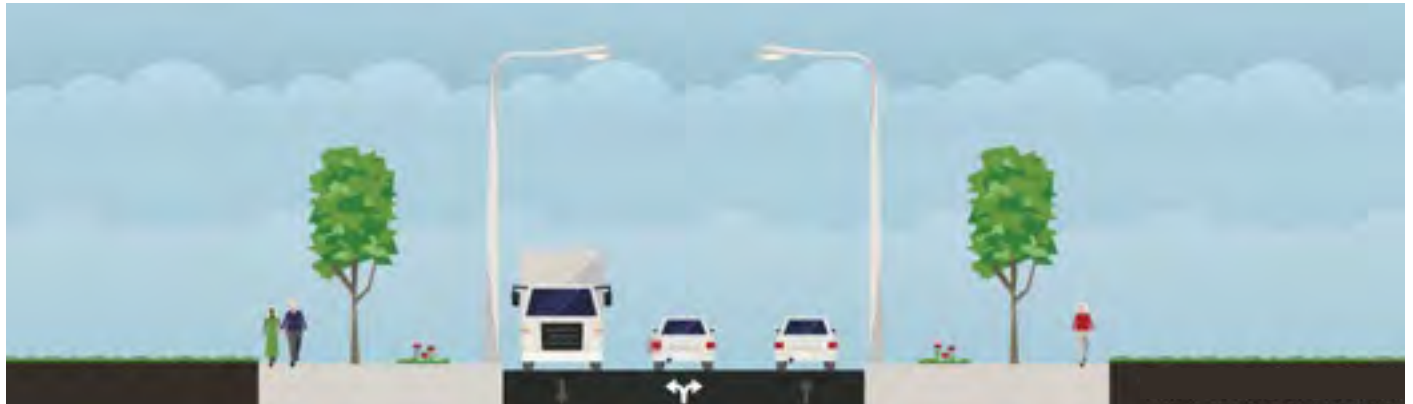
▼ FIGURE 1.8 EXAMPLE OF THREE-LANE ROADWAY CROSS-SECTION Source: City of Rock Hill Planning & Development and Streetmix.net
