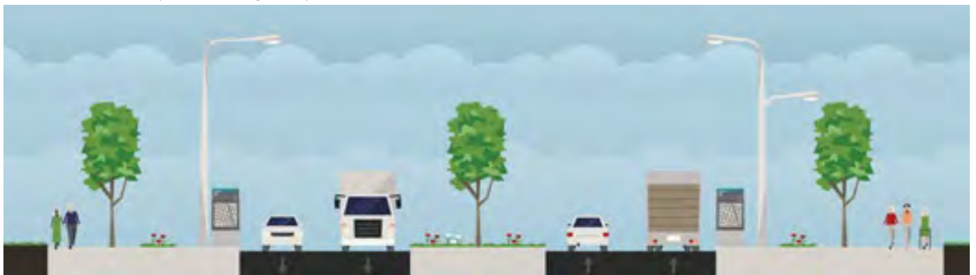
▼ FIGURE 1.9 EXAMPLE OF FOUR-LANE DIVIDED ROADWAY CROSS-SECTION Source: City of Rock Hill Planning & Development and Streetmix.net
